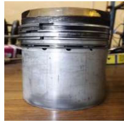
Photo Graphic View of Aluminium Piston with Brass Crown and Air Insulation
